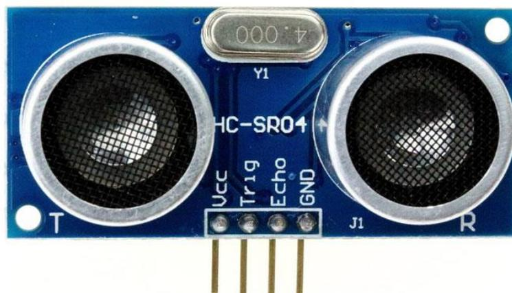
Gambar 5. Sensor Ultrasonik HCSR04
